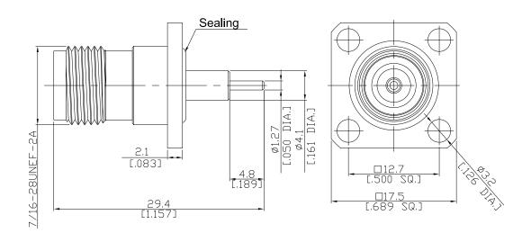
All dimensions are in mm [inch] Tolerances according to DIN ISO 2768-mH
