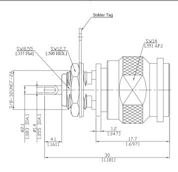
All dimensions are in mm [inch] Tolerances according to DIN ISO 2768-mH
