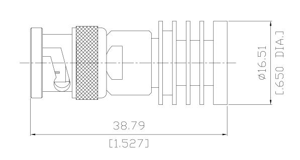
All dimensions are in mm [inch] Tolerances according to DIN ISO 2768-mH
