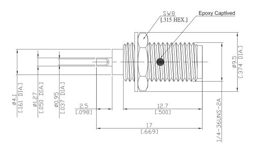
All dimensions are in mm [inch] Tolerances according to DIN ISO 2768-mH
