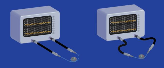
▲ Wrapped a full 360° around a mandrel of 57 mm (2.25 in) diameter.
