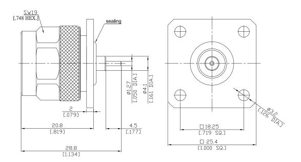
All dimensions are in mm [inch] Tolerances according to DIN ISO 2768-mH
