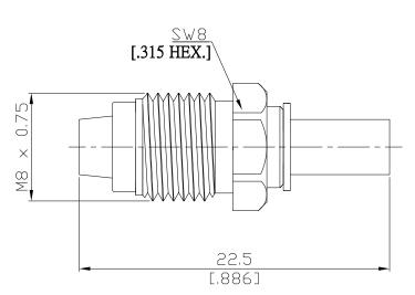
All dimensions are in mm [inch] Tolerances according to DIN ISO 2768-mH
