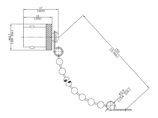
All dimensions are in mm [inch] Tolerances according to DIN ISO 2768-mH
