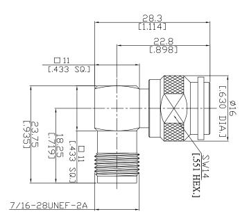
All dimensions are in mm [inch] Tolerances according to DIN ISO 2768-mH
