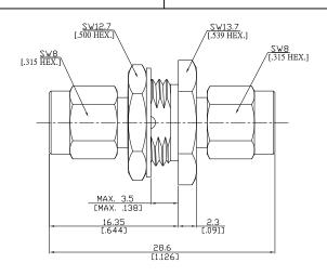
All dimensions are in mm [inch] Tolerances according to DIN ISO 2768-mH
