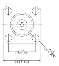
All dimensions are in mm [inch] Tolerances according to DIN ISO 2768-mH
