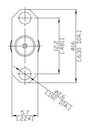
All dimensions are in mm [inch] Tolerances according to DIN ISO 2768-mH
