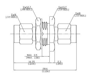
All dimensions are in mm [inch] Tolerances according to DIN ISO 2768-mH
